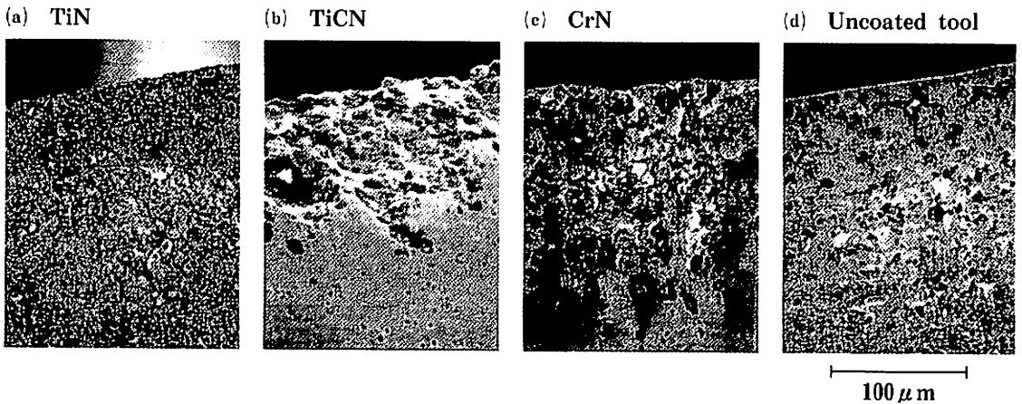
Figure 6. SEM micrographs of the rake faces for all tools in cutting at an electrical-potential of  $+1$  kV (anode voltage)
