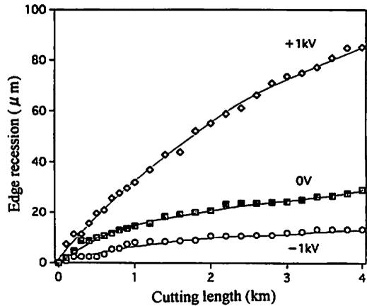
Figure 7. Progression of tool wear and changes in electric-current flow during cutting where increases in cutting length
