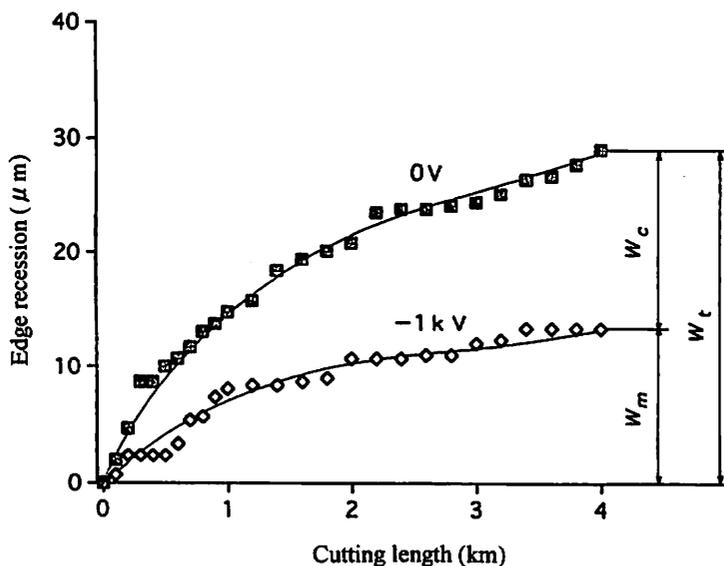
Figure 9. Wear mechanism of a cutting edge in the cutting of high moisture-content wood consists of mechanical wear and corrosive wear.  $W_t$ , edge recession under electrical-potential of 0V in normal cutting;  $W_m$ , mechanical wear;  $W_c$ , corrosive wear ( $W_c = W_t - W_m$ )
